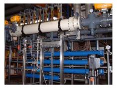
As opposed to microfiltration, in reverse osmosis no porous ("permeable") membranes are in charge of separation and/or transport, which means that the solvent is transported through the "leak-proof" membrane by means of solution-diffusion processes. Reverse osmosis (RO) is a membrane process for separating solutes (salts, macromolecules) from a liquid. In reverse osmosis, the osmosis principle is reversed.
